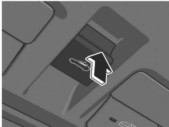
2. Press the tilt/slide switch forward 2 times.
