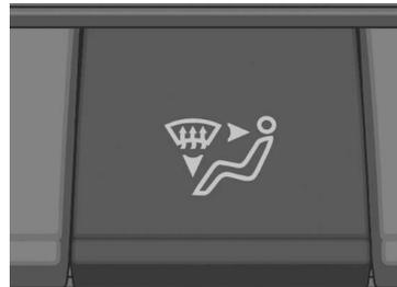
The desired airflow mode can be selected. The mode changes each time the switch is pressed. The selected mode is indicated on the display.
