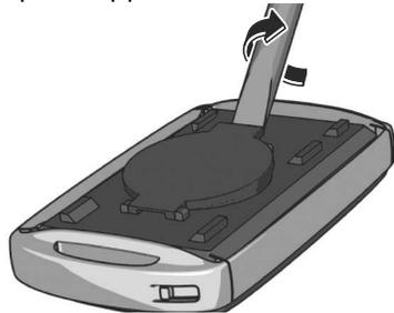
6. Remove the battery using the tape-wrapped flathead screwdriver.
