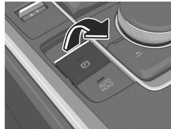
When the shift-linked release is enabled, a sound is activated 2 times, the EPB switch indicator light switches to fast flashing, and then flashes for a certain period of time. When the shift-linked release is disabled, a sound is activated 1 time, the EPB switch indicator light
