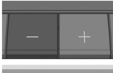
The airflow amount changes each time the switch is pressed. The airflow amount is indicated on the display. The airflow amount can be adjusted to 7 levels.
