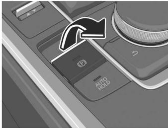
The parking brake is applied and the EPB indicator light <sup>(P)</sup>PARK in the instrument cluster and the EPB switch indicator light turn on.
