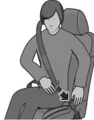
5. The belt should fit the pelvis as low as possible.
