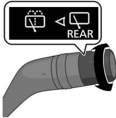
While the switch is in the
