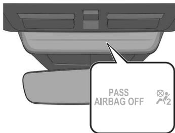
If the front passenger weight sensors are normal, the indicator light illuminates when the vehicle power is switched ON. The light turns off after a few seconds. Then, the indicator light
