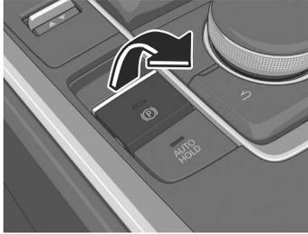
The brakes are applied and the vehicle can be decelerated/stopped.
